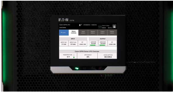
Green light bars showing healthy UPS.
